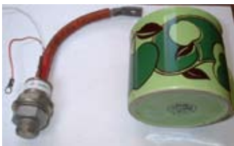
SCR-Silicon Controlled rectifier-hi-voltage-for industrial robotic computerized machine
