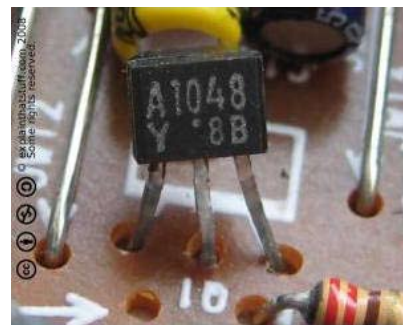
Transistor component soldered on board
